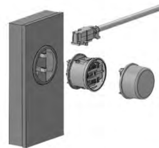
Plug-in adapter uses meter socket instead of the service panel
